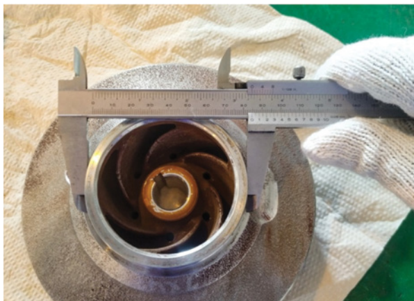
FIGURE 2. A mechanic inspects a centrifugal pump impeller during a repair
