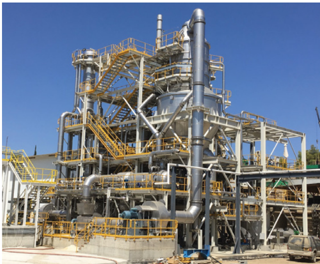
FIGURE 1. Due to crystallizers' unique abilities to deliver high-purity chemicals, they are being frequently deployed to purify critical battery materials, such as nickel sulfate hexahydrate
